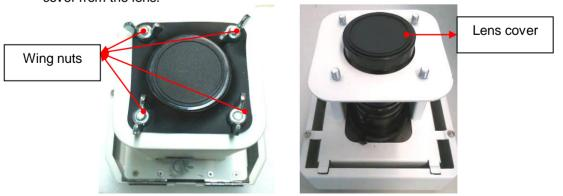
**3. Mount Camera Holder:** Align the shielding rubber on top of the darkroom. Place and align the camera holder to the four screw holes on top of the darkroom unit.
