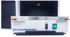
c. Insert the short side of the protection cover into the support holder as followed picture.
