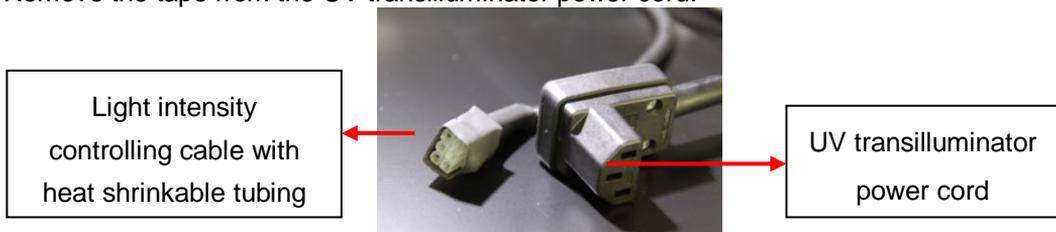
Position the UV transilluminator on the sliding frame of the darkroom with the UV transilluminator power switch facing the installer. Inside the darkroom unit, plug the UV transilluminator power cord to the UV transilluminator AC socket and light intensity controlling cable nearby at the rear side of the UV transilluminator.
