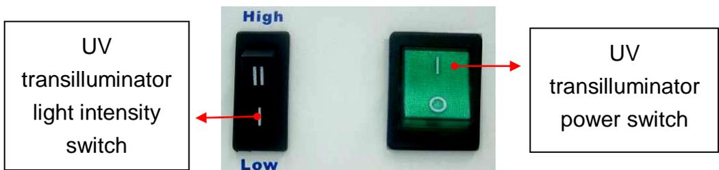
**Note:** When the MD25K is used in the KETA series imaging system, the light intensity switch should be switched to “Low” in order for the Magic 1D to control the light intensity switching.
