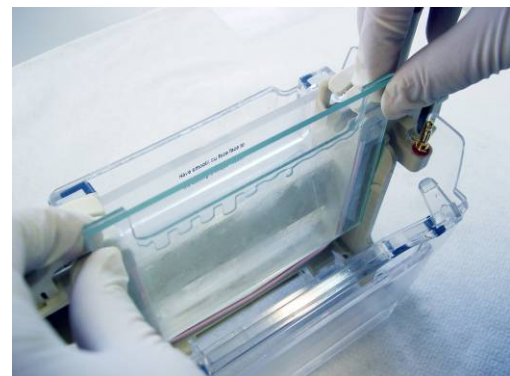
Figure 9. Insert the glass sandwich into the electrode module. Slide the sandwich closely along the pink silicone rubber on the middle part of the module making sure the inside of the gel sandwich rises.
