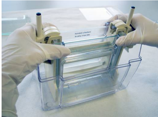
Figure 10. Press together the doors of the electrode module. A clicking sound indicates that the doors are securely locked. When opening the lock, press down both sides of the white clamp-releasers (4 pcs) and slide the gel upwards.
