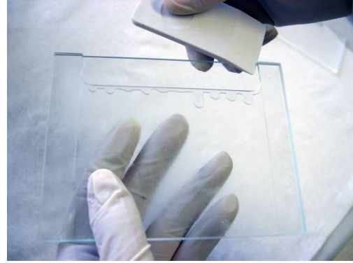
Figure 14. Separate the glass plates using the glass plate separator. Wiggle carefully at one corner until the glass plates separate.
