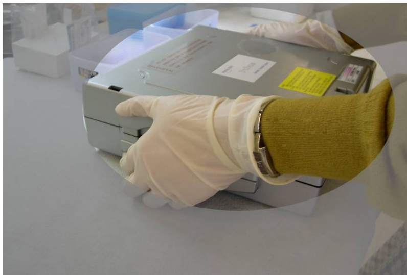
Figure 7: With both hands, apply equal force to both sides of the blotter and press together (Same procedure as for unlocking after transfer).
