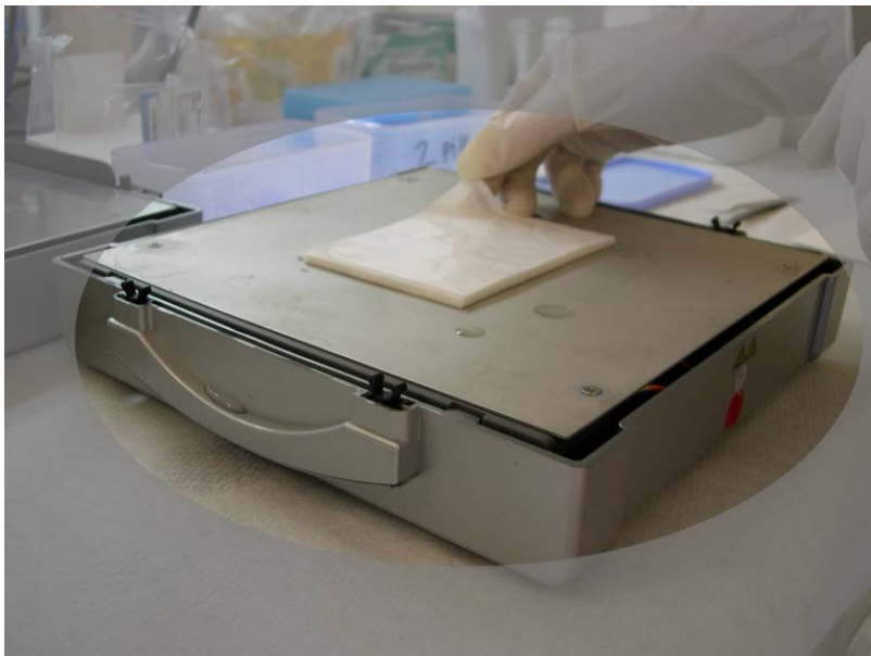
Figure 3: Position the wet membrane on top of the filters.
