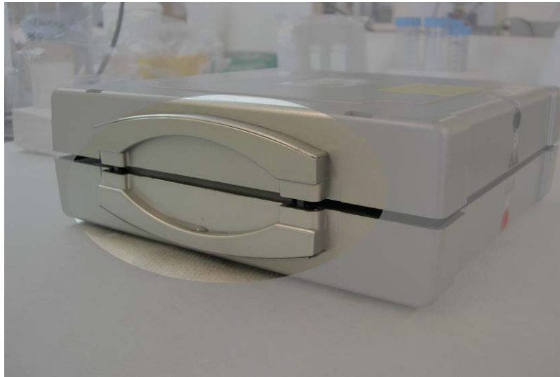
Figure 8: When the plates are correctly adjoined, the gap between the plates is equal all around the blotter. The adjoining points are not visible.
