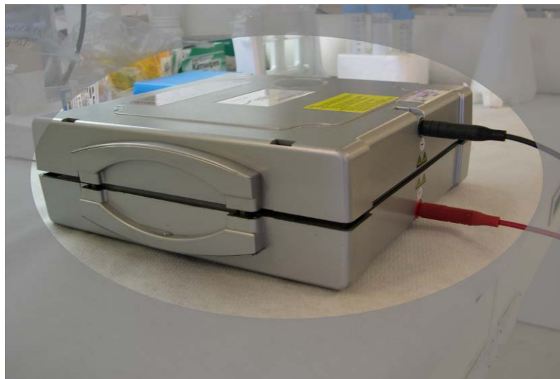
Figure 9: Connect the electrode wires to the power supply and start transfer.
