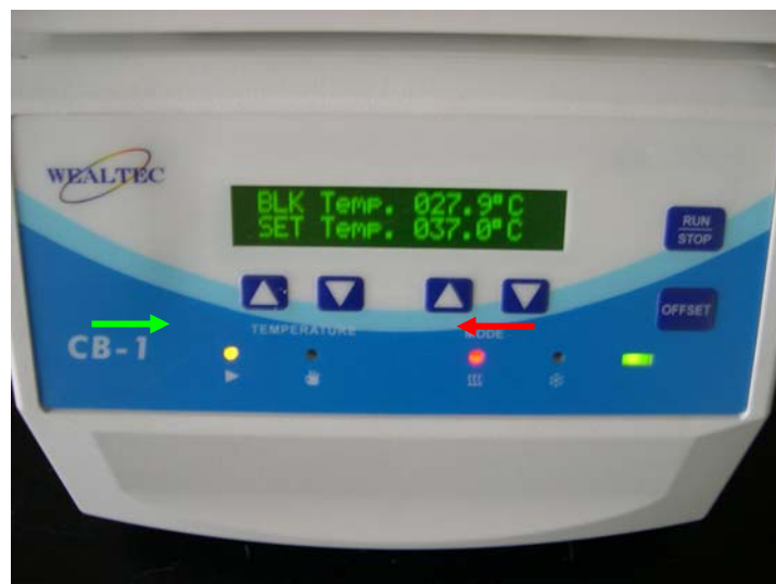
Figure 3: The display will show the set temperature (SET), as well as the current block temperature (BLK). When in heating mode, the red "heat"-indicator (red arrow), as well as the "power"-indicator (green arrow) are lit.
