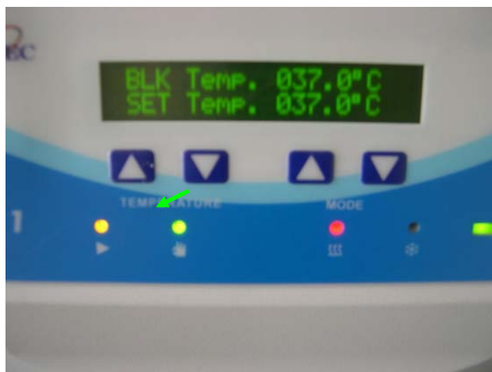
Figure 4: When the target temperature has been reached, as indicated by the display and the green "ready"-indicator glowing steadily (green arrow), the block cooler is ready to be used.
