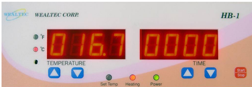
Figure 2: Once the block heater starts warming up, the left display will show the current temperature and the “Heating”. The power indicators will be lit.
