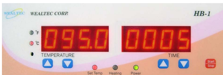
Figure 4: Set the timer by pressing the “Up” and “Down” buttons below “TIME”. To start the timer, press the Stop/Start button.
