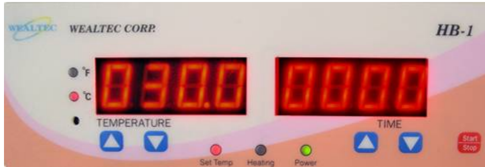
Figure 1: Set the temperature by pressing the “Up” and “Down” buttons (green arrows) below “TEMPERATURE”. The “Set Temp” and the Power indicators will be lit. The set temperature is shown on the left display. Press the “Stop/Start” button (blue arrow) to start warming the unit.
